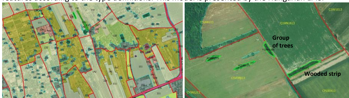
Figure 1-3: The Hungarian example of categorizing LCC elements of a continuous LPIS layer for selection of LFs among non-eligible areas of LPIS physical blocks, based on different land cover categories, adjacency rules and average and min/max size limits 1 . Left image: Red lines: physical block boundaries, cyan spotted: non-eligible area, semi transparent shaded: different land cover categories inside the PBs. Right image: light green boundary: woody LFs, yellow numbers: PB IDs.
