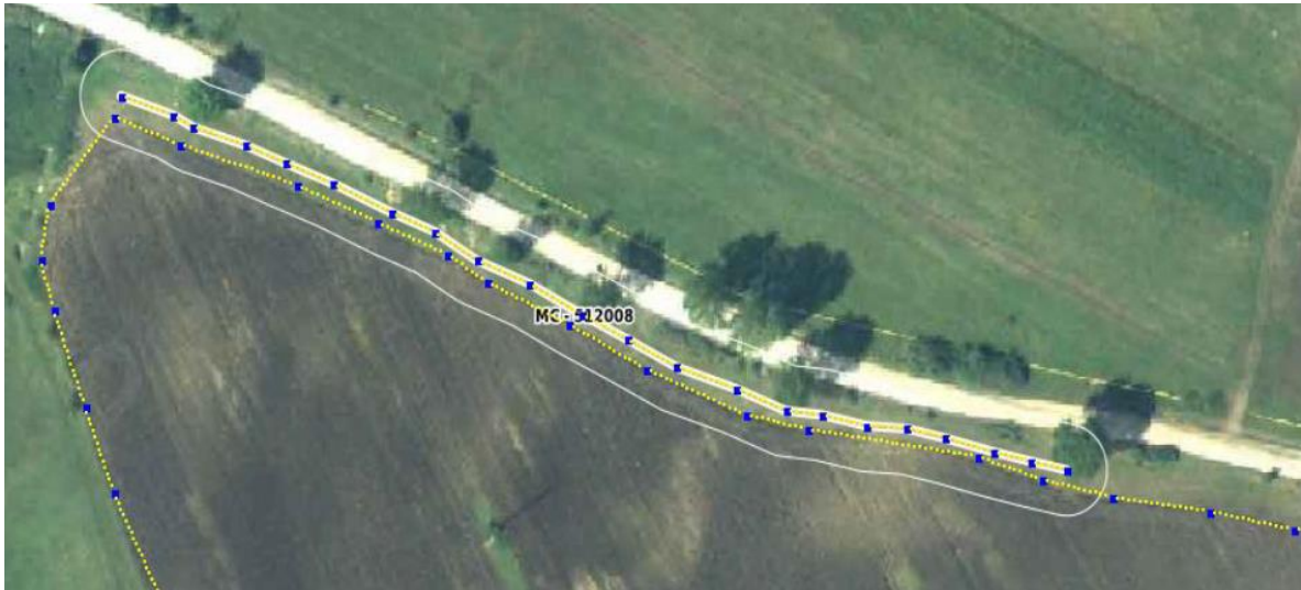
Figure 2-5 Example of a field margin delineated on orthophoto images with a line using the line tool of the IPA - Online GSAA application.
