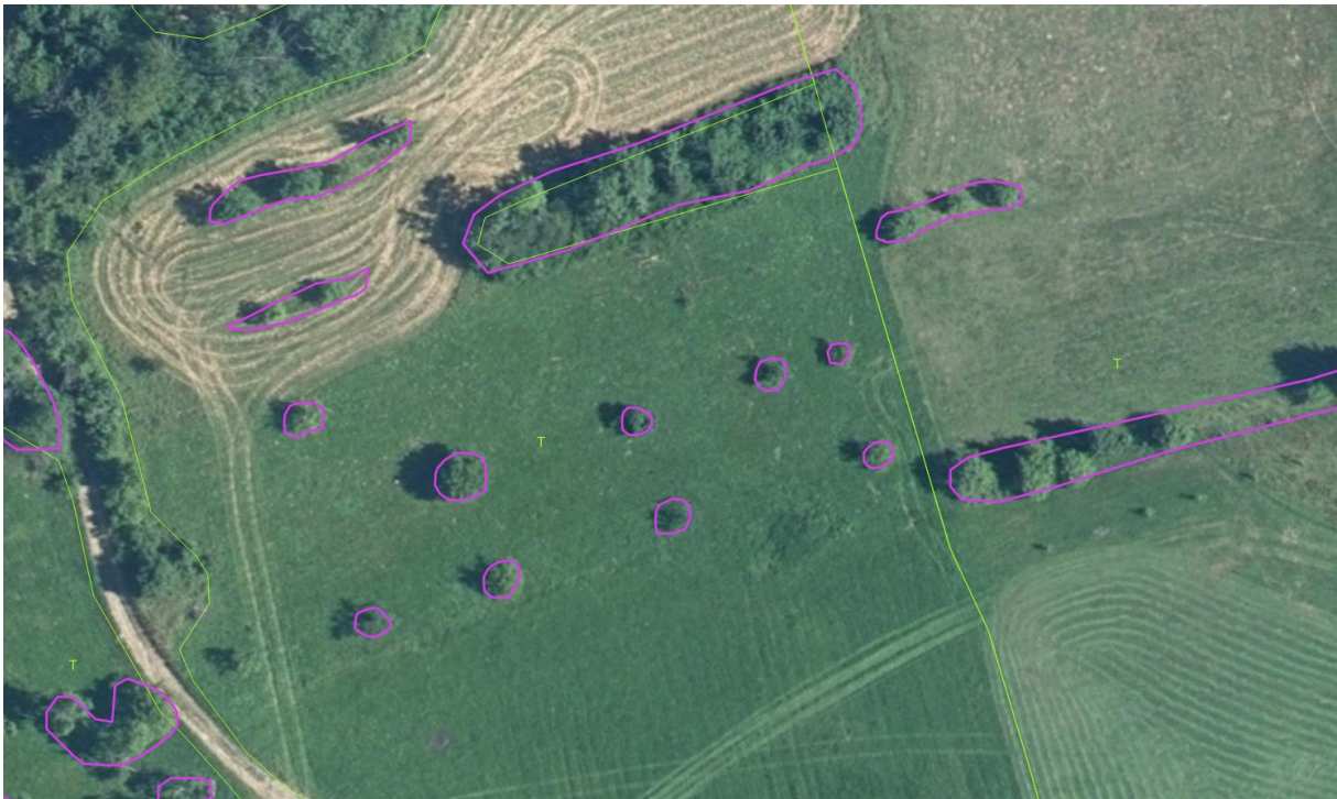
Image 3. Example of vectorisation of Isolated trees according to the border of their tree crowns
