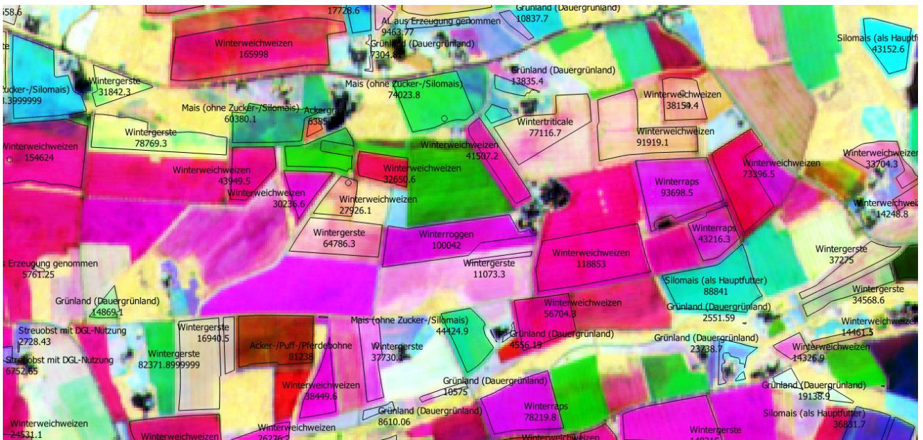
Image 6. False color composite in y2020 to visualize the NDVI stack where R = NDVI\ 2020.05.07 , G = NDVI\ 2020.09.19 , B = NDVI\ 2020.03.23
