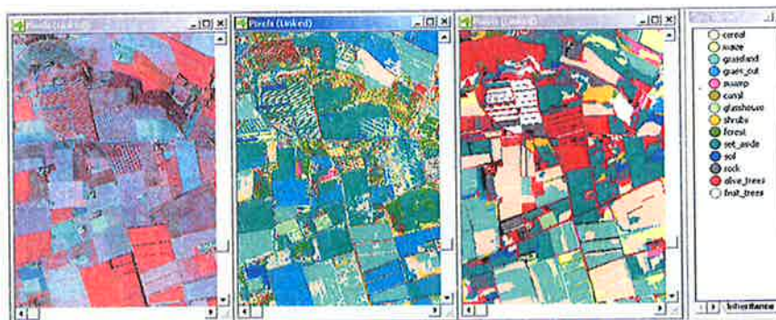
'Les Alpilles' site from left: cc ADS40;/ ADS40 mic based on Frost filter 7x7; // QB classification ecogn 150 sc, spectral m,stdev, ratio
