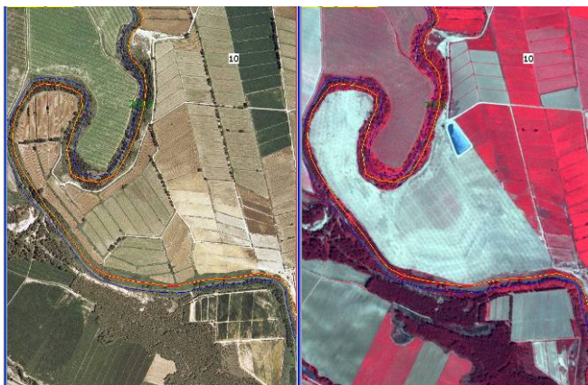
Figure 2. STANDARD GAEC08. Difference between orthophoto and current year VHR image.
