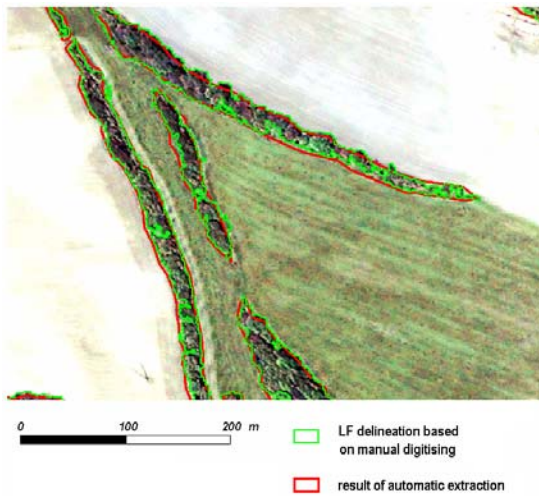
Figure 6: LF delineation as a result of manual digitising compared to automatic extraction
