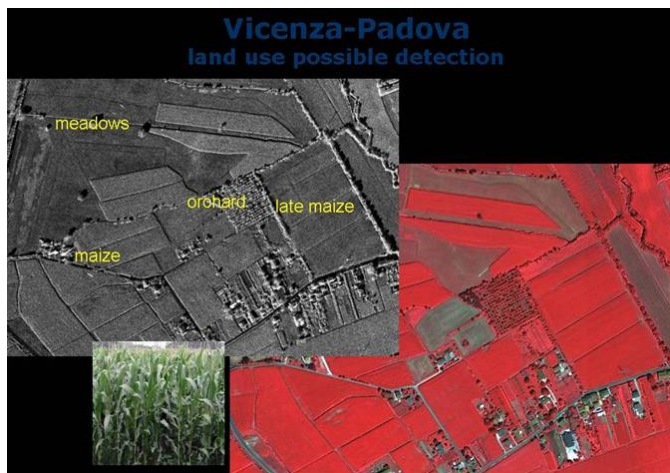
Fig. 6: Land use detection by SAR, through geometric features
