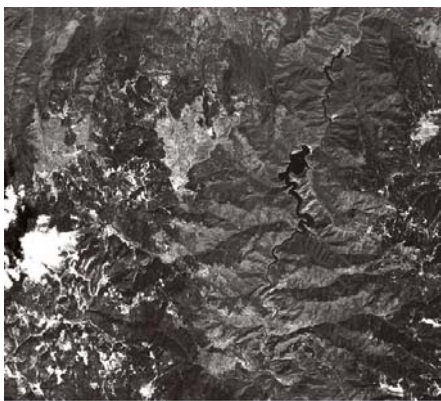
Figure 5. Panchromatic orthoimagery from the HRS sensor with a spatial resolution of 5 meters, part of the Reference 3D product.
