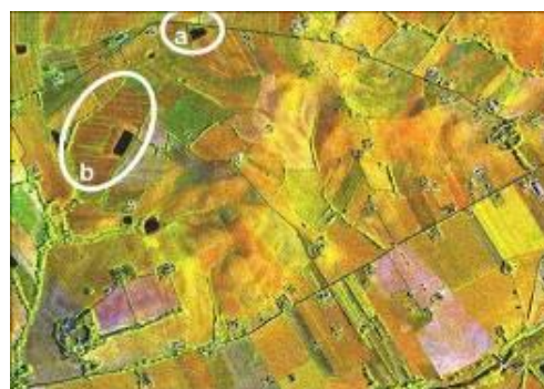
Figure 4 Coherent MultiTemporal false colour composite RGB done over the Macerata area realized through a COSMO-SkyMed Spotlight-2 interferometric couple; highlighted the changes on the water level of the reservoir (a) and on the ditches status [RED: SAR detected amplitude of the first acquisition (17/11/2008), GREEN: SAR detected amplitude of the second (05/02/2009), BLUE: interferometric coherence]
