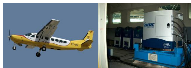
Figure 1. ICC Cessna Caravan B208 airplane (left) and DMC sensor (developed by Zeiss / Intergraph Imaging) for obtaining images (right).
