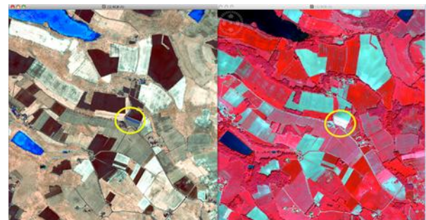
Figure 22. Combination of Vegetation Indices (RGB) versus False Colour Composite. Left: ARI2-NDVI RE -ARVI RE -Co.; Right: classical FCC (RGB): NIR1-Red-Green.
