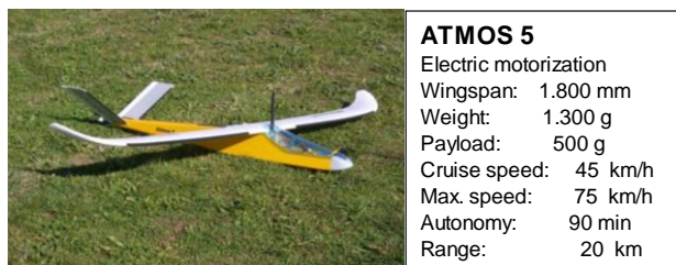
Figure 2. Image of the ATMOS 5 UAV and its characteristics.
