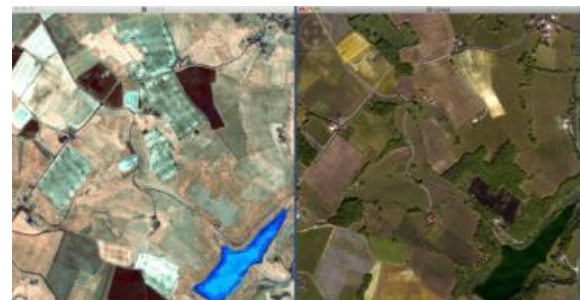
Figure 23. Combination of Vegetation Indices (RGB) versus True Colour Composite. Left: Veg. Index combination (RGB): ARI2-NDVI RE -ARVI RE -Co. Right: “enhanced” TCC (RGB): Yellow-Green-Coastal (all bands previously enhanced)
