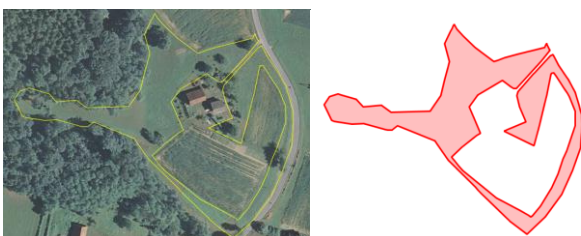
Figure 15. An example of a large (1 ha) parcel, which looks normal but is quite long based on perimeter area/ratio
