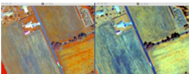
Figure 26. Comparison pan-sharpened with multi-spectral data (same band combinations: NIR-1, Red Edge, Green). On the left: image pan-sharpened, on the right: original multi-spectral.
