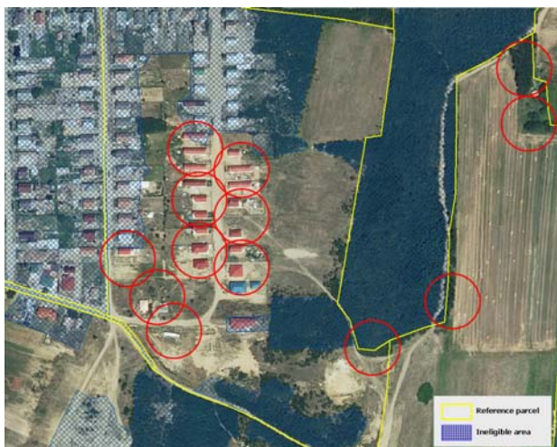
Figure 3. The state of the LPIS in the year 2007, the LPIS layer for the reference year for 2007 overlaid with up-to-date ortho-image acquired using Ultracam D (AOI1).
