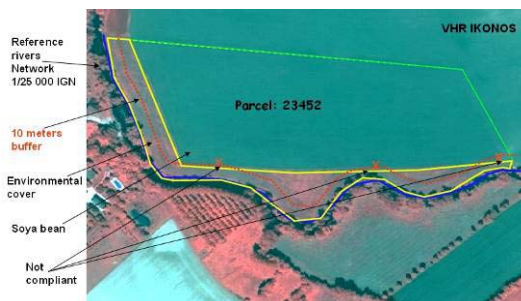
Figure 7: Example of superimposition of a river network layer on a VHR Ikonos image to automatically check the compliance of a 10 meters width buffer strip of ‘green’ cover along water courses.
