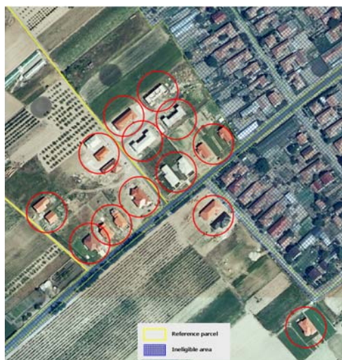
Figure 6. The state in the year 2007, the LPIS layer for the reference year 2007 overlaid with up-to-date ortho-image acquired using Ultracam D (AOI2).
