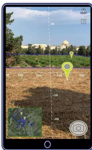
Figure 11: "SITI Land AR" App facilitating geotagged imagery capture. Augmented reality is used to direct the user to the targeted parcel with camera tilting, parcel borders and parcel identifiers displayed real-time (Courtesy of Abaco Company, IT).
