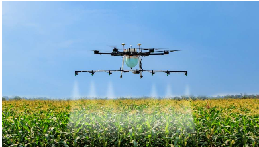
Figure 5: UAV used for precision Plant Protection Product spreading over a corn field
