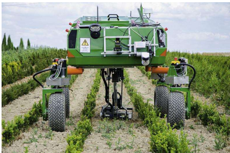
Figure 3: 'Bonirob' robot developed by Deepfield Robotics to automatically pick out weeds in crops
