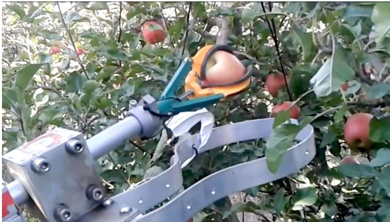
Figure 2: Test of automatic apple harvesting by FFRobotics Company
