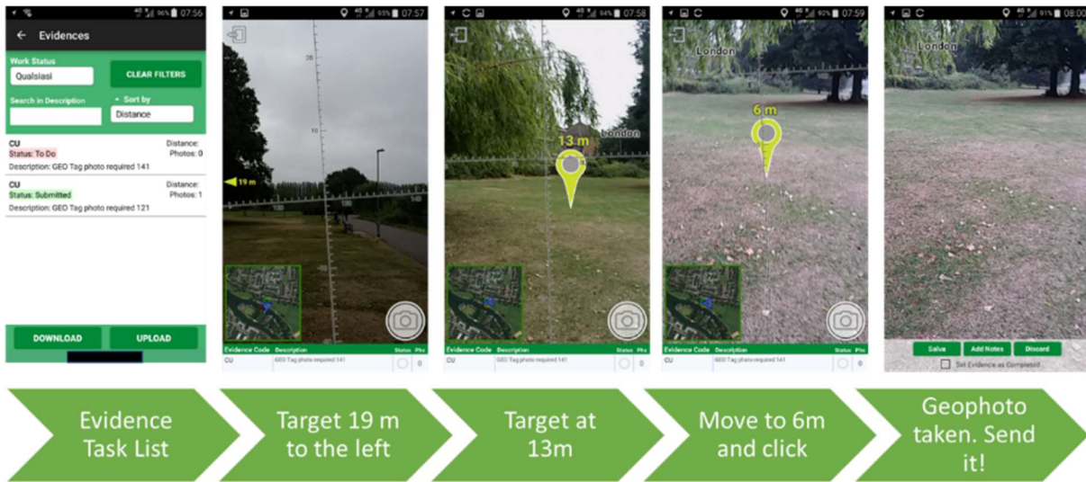
Figure 5. ABACO GEOPHOTO: typical geotagged image acquisition workflow (with augmented reality). After receiving a task, the user is navigated to the point from which the photo should be captured. The current device position and the parcel with the target point are shown on an overview ortho-photo map. The number of photos collected for this task is also made visible. Once the geotagged photo is taken a note can be attached.
