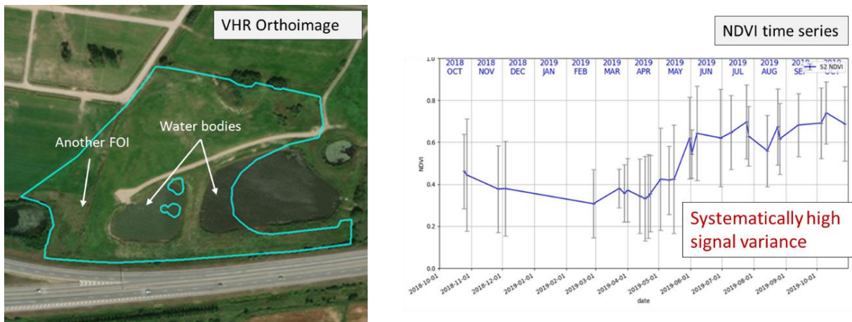
Figure 3: Issues with spatial cardinality propagating a noise in Sentinel signal used in CbM
