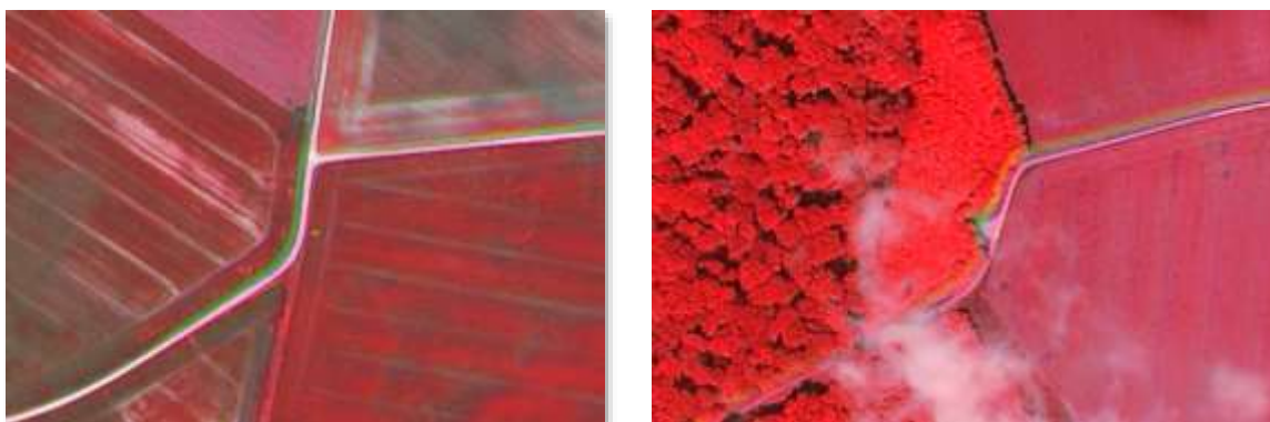
Figure 18 - RED band misalignment detected during image Quality Control (QC).
