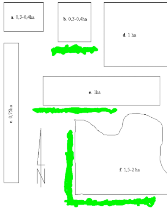
Figure 4: Example parcel configuration scheme for GPS measurement system validation. Obstructions of the horizon marked in green. (Oszczak and Ciecko, 2007)
