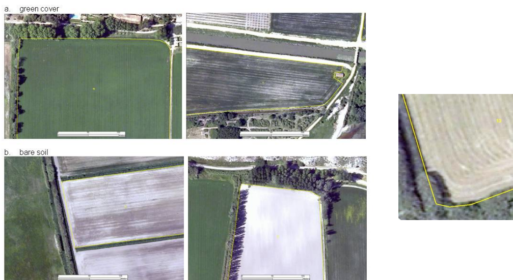
Figure 5: Example of the graphical illustration of the digitization key defined for different land covers (Pluto-Kossakowska, 2008)
