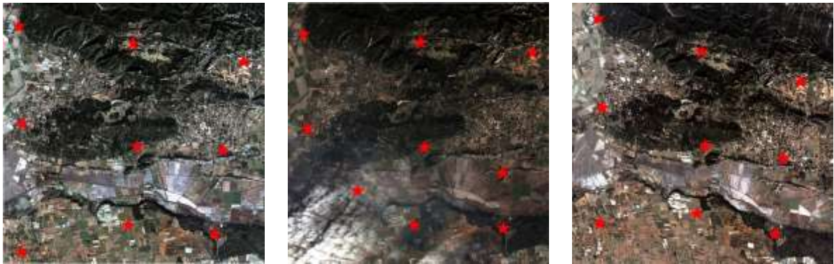
Figure 7: Localisation over the primary images of the GCPs used for orthorectification. From left to right: GCPs selected over Maussane test site for the 4°, 22° and 30° images resp. (red star F, at most 9 for each image). See also Figure 6.
