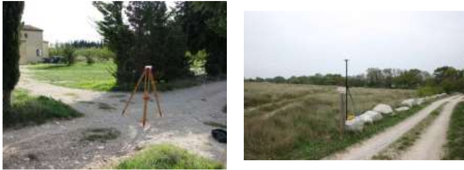
Figure 4: Example of ground camera shots of GCPs positioning. The ground accuracy of some of the GCPs used for orthorectification (GCPs #1 and #7 are displayed here) can be challenged.
