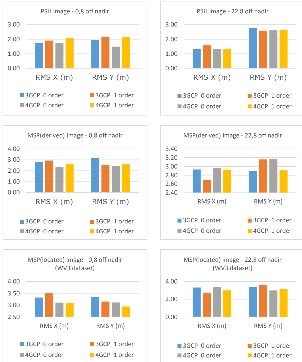
Figure 31 Graph representation of RMSEs comparison between orthoimages produced using 0 RPC order and 1RPC order, PCI software.
