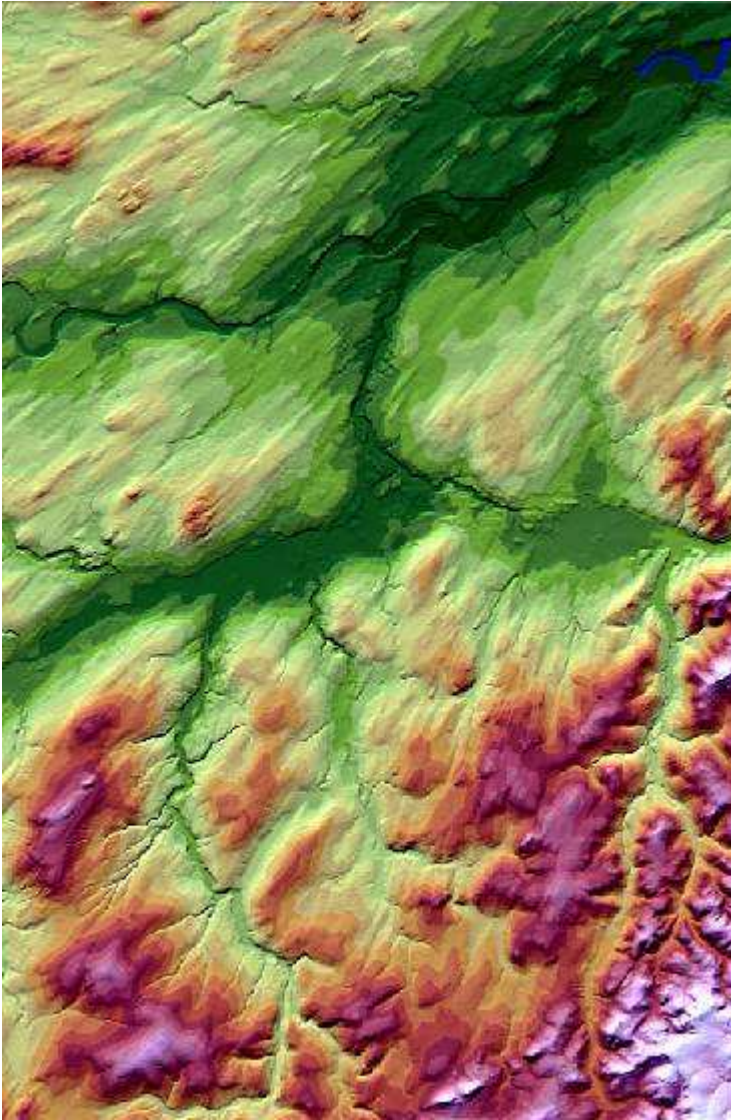
Fig. 5 Extract of the DEM over LPIS control zone RS02 (shown as painted relief)
