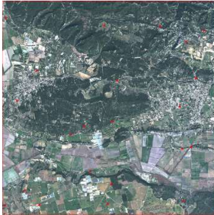
Figure 14. ICPs dataset used by JRC in the EQC of PNeo ortho imagery.
