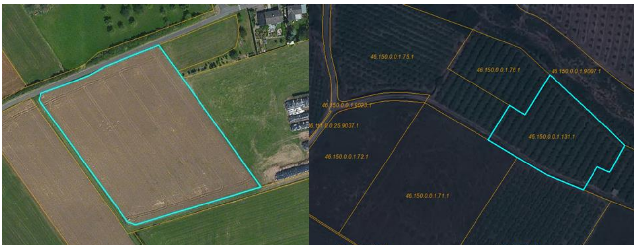
Figure 6. Two examples of clipping: left - clipped "observation boundary" matches the LUI, right - clipped "observation vector" ignores the road in the south, the resulting observation is manifestly incorrect but enters the data processing.
