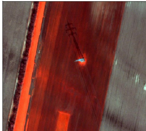
Example 4: Visible electric poles with artificially sealed surface inside RP perimeter. If observed area is conforming than the contamination occurrence should be counted for QE2a.
