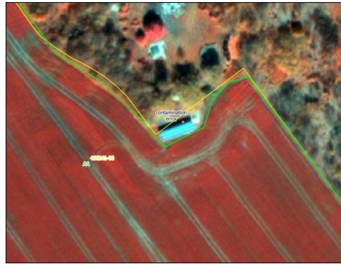
Example 2: Visible built up construction inside RP perimeter. It is an area conforming parcel but contamination occurrence should be counted for QE2a. (yellow line is the LPIS RP polygon)
