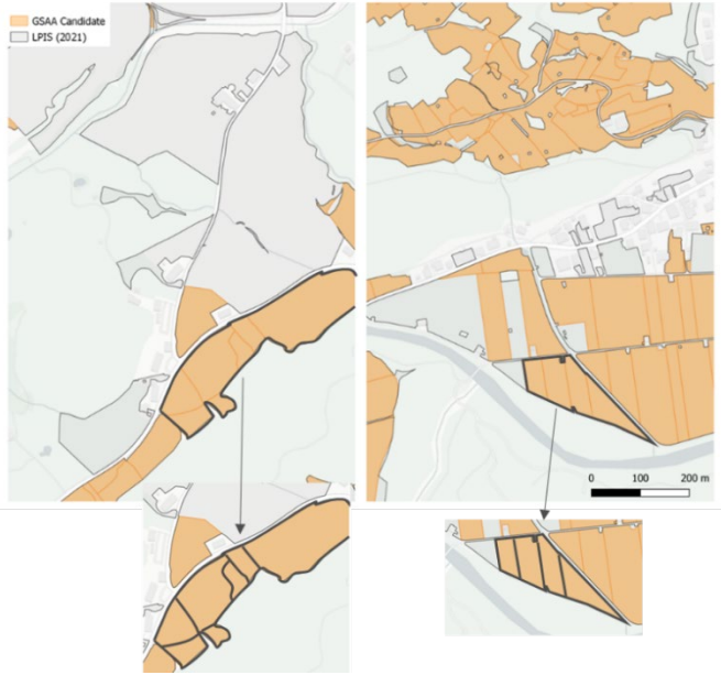
Figure 14. Geometrically stable GSAA parcels (yellow borders) superimposed on the LPIS parcel layer (black borders), with the proposed LPIS updates at the bottom of the figure.
