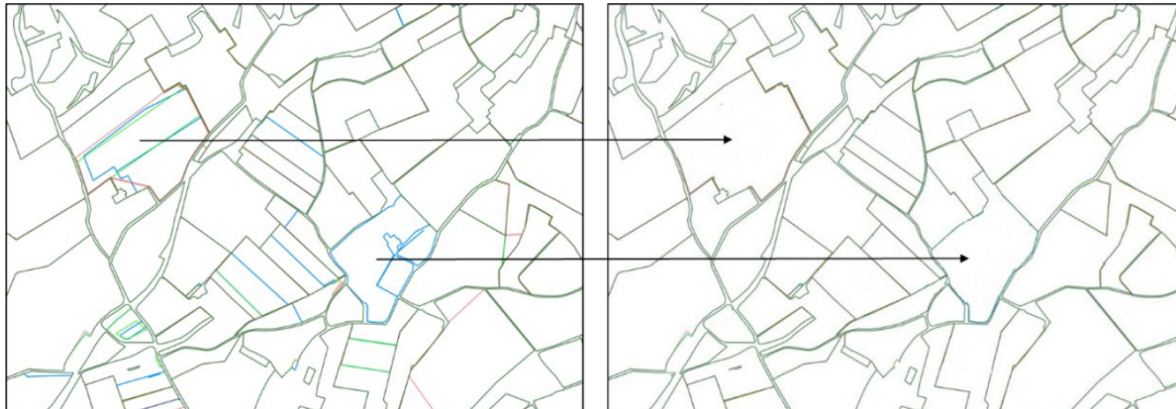
Figure 15. Identification of candidates for a Reference Parcel layer (right) out of the overlay of three consecutive years of GSAA (left) (2018 in Red, 2019 in green and 2020 in blue). Limits non-permanent over three years are dissolved to keep stable limits as candidate RP.
