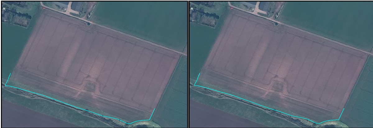
figure 4e.2: original (left) and georeferenced (right) survey vector. The survey vector is translated.
