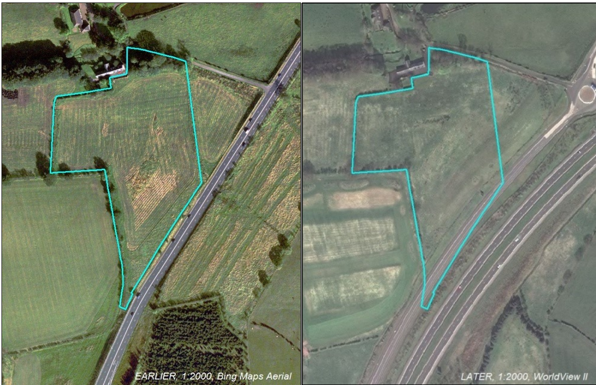
Figure 9: Irreversible conversion of agricultural land. Appearance of roads. In this case the new construction pushes the existing road into the reference parcel.
