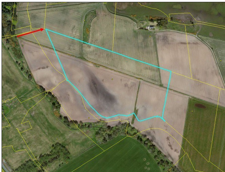
Figure 10: A typical shift between reference parcel layer and orthophoto caused by different use of CRS
