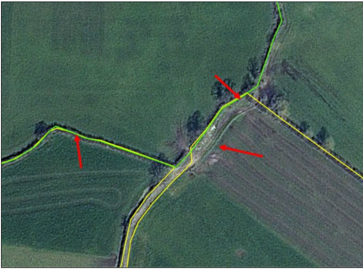
Figure 5: Example of gaps and slivers within the 'RP layer' in the system
