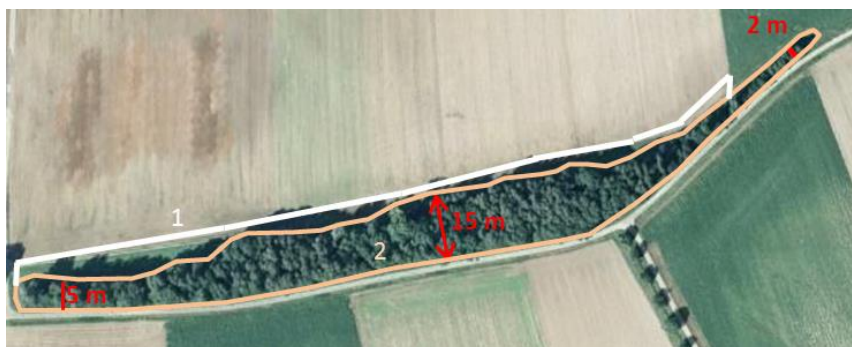
Figure 4-5 – The width of the hedge (2) varies between 2 m and 15 m. In this case, the average width should be noted, in this example this would be 10 m.
